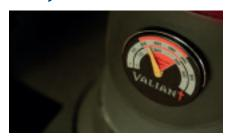
Keep it hot, if you are using a flue thermometer, aim for the middle of "best operation"
